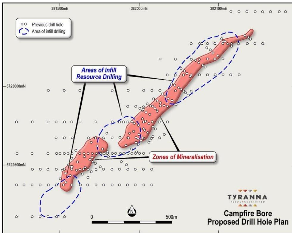
Figure 1: Campfire Bore proposed drill hole plan
