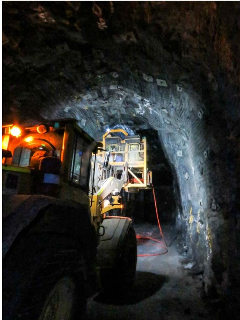
Figure 1: Stope prepping and charging in the 115 M2S2 Right drive – Challenger Deeps
